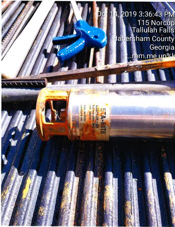
Pump that was removed from the well indicating it to be 30/gpm – 5/hp larger than what was approved by the EPD.
