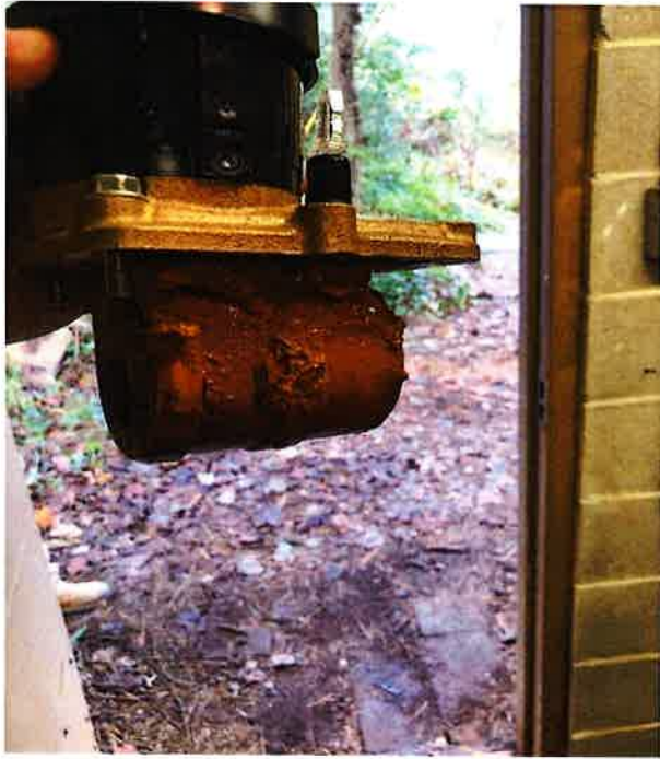
This is a side picture of the meter head showing the iron sludge.
